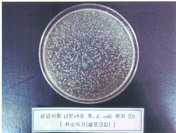
Bactericidal test (after 2 min ± 5 s, E. coli , test position ① ) [ Book Sterilizer (Self Clean) ]
