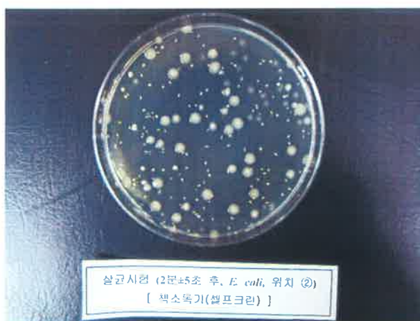
Bactericidal test (after 2 min ± 5 s, E. coli , test position ② ) [ Book Sterilizer (Self Clean) ]
