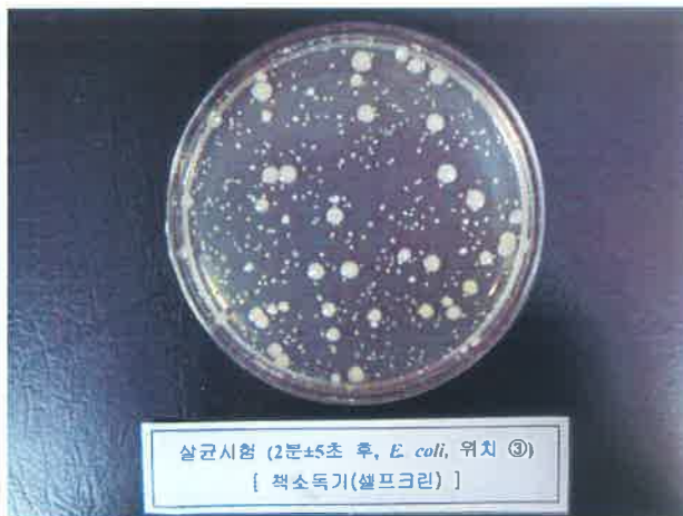
Bactericidal test (after 2 min ± 5 s, E. coli , test position ③ ) [ Book Sterilizer (Self Clean) ]
